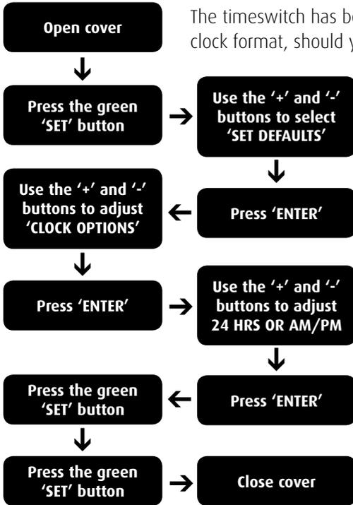
The timeswitch has been preset to display the time in 24 hour clock format, should you prefer AM/PM format then please use the procedure given in the flowchart opposite.
