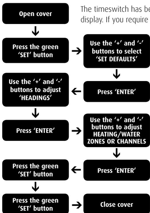
The timeswitch has been preset without a channel heading on the display. If you require either the 'Water' or 'Heating' options then please follow the flowchart opposite.
